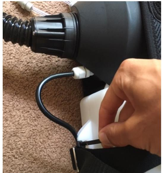
5. Repeat with a second zip tie at the bottom of the tank slot. Make sure to not pinch the backpack strap. Ensure the backpack strap can be tightened and loosened.
