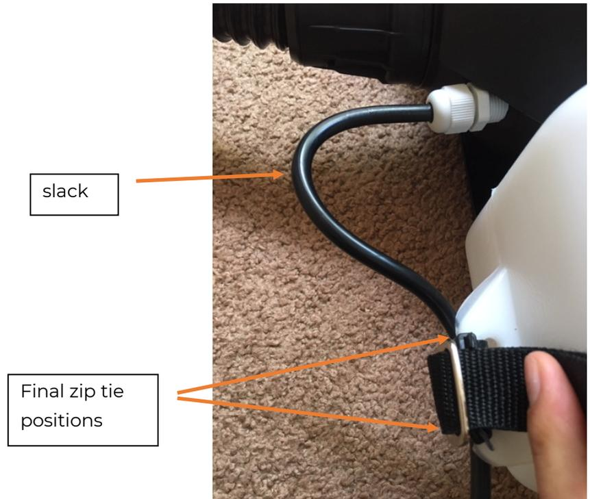
2. Hold power cord against tank ledge being sure to leave slack between the cable gland and the tank.
